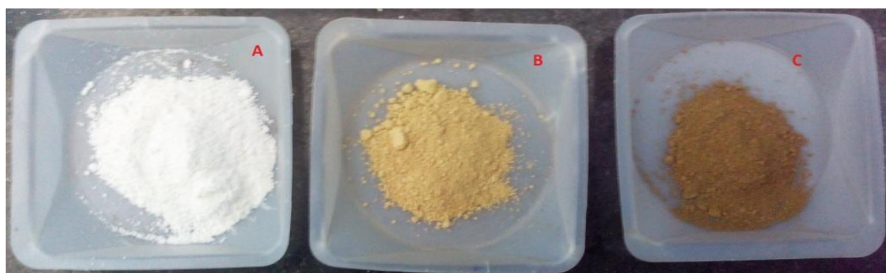
Figure 1: As-synthesized ZnO (A), Ag/ZnO 1 (B) and Ag/ZnO 2 (C) nanoparticles
