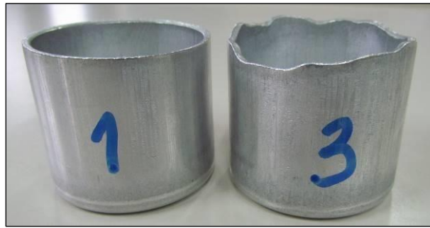
Fig. 2. Cartridge cases without (1) and with earrings (3).
