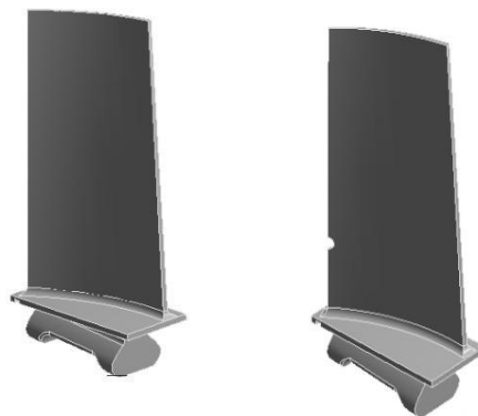
Fig 1: Twisted turbine blade with and without notch.
