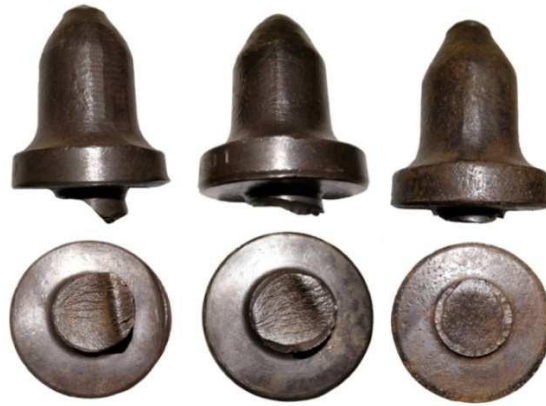
Fig. 3. Examples of the point-attack pick with low tip wear and fatigue broken shafts in the transition area between the shank and the shoulder
