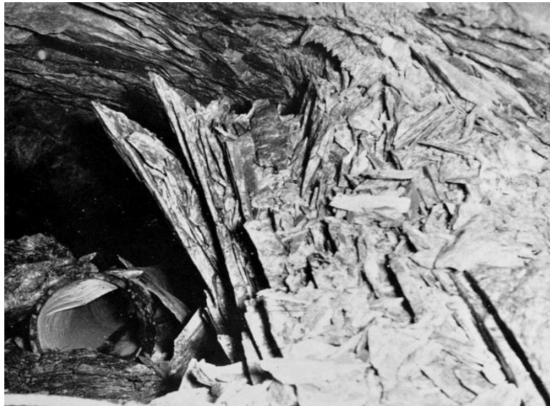
Figure 1. Effects of a rockburst in a deep-level South African gold mine.
